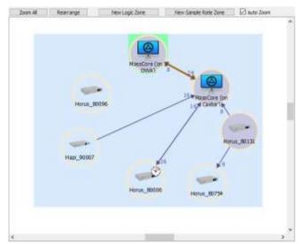
Devices appear in the world view if they are discovered on the network. All Ravenna devices will show in the view but only supported devices will be fully controllable with the software.
