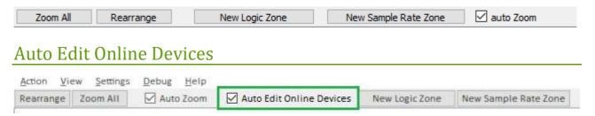
The Auto Edit Online Devices option will automatically detect all the online devices and populate the Matrix, and has been designed for small scale configuration.
